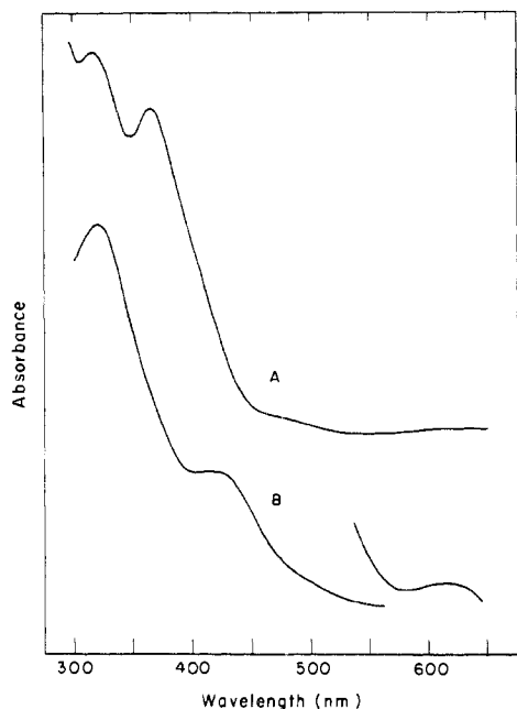
Figure 2. Visible spectra of (A) [\text{Co}((c\text{-Hx})_2\text{dtc})_3] and (B) [\text{Co}((c\text{-Hx})_2\text{dtc})_3]\text{BF}_4 in methylene chloride solution.
